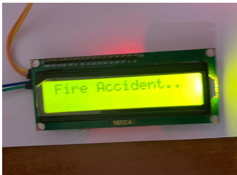
Figure.6 Fire detection On LCD
