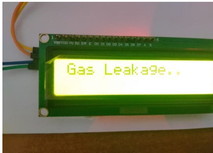
Figure.4 Displaying Gas leakage On LCD
